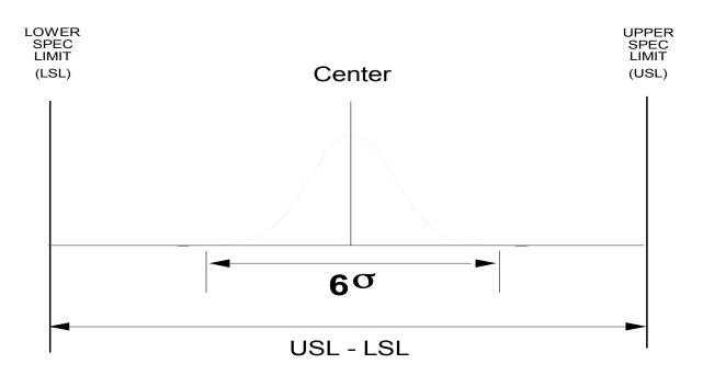
Although the distribution shown above is "centered" (average = mid point of the specification range), note that the equation for  $C_p$  is dependent only on the specification width (USL - LSL) and process width ( $6\sigma$ ). As such, it does not depend on the location of the distribution.
