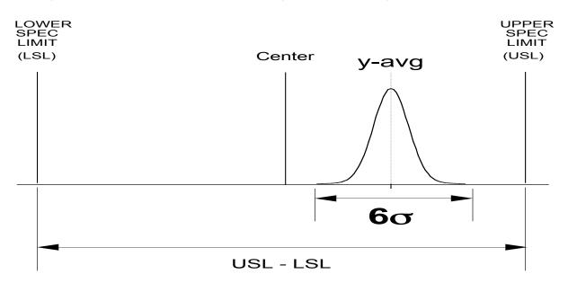
In this situation, process capability is defined by a calculation which takes into account the effect of the off-set of the process average from the center of the specification range.
